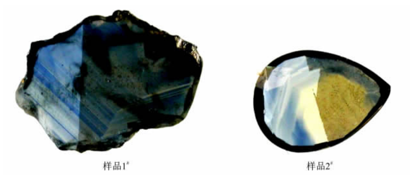
图 1 经过 Be 离子注入处理的山东蓝宝石样品(右侧区域经 Be 离子注入处理) Fig. 1 Sapphire samples from Shandong Province treated by Be (right: treated)
