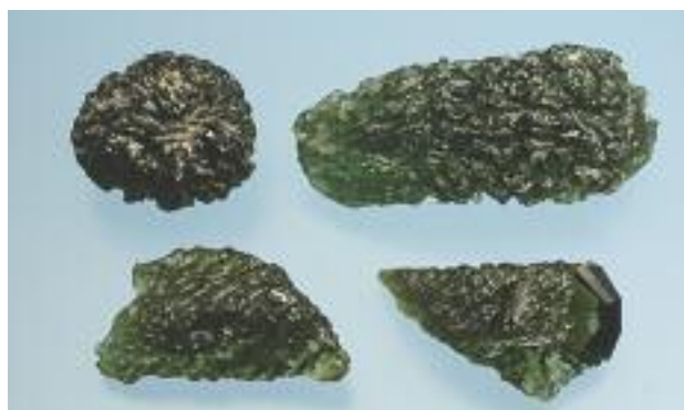
Figure 14. Two moldavites from southern Bohemia, Czech Republic (top row) and two recent imitations from China (bottom row). The natural specimen on the top right measures 44 mm across. Photo by Jaroslav Hyršl.
