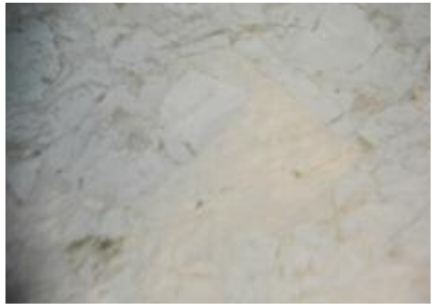
Figure 11. Two groups of minerals were observed on the surface of this sample under brightfield illumination. One group is composed of the pale whitish subhedral to euhedral grains, the other of the creamy minerals in between. Photomicrograph by Li Jianjun; magnified 30 \times .
